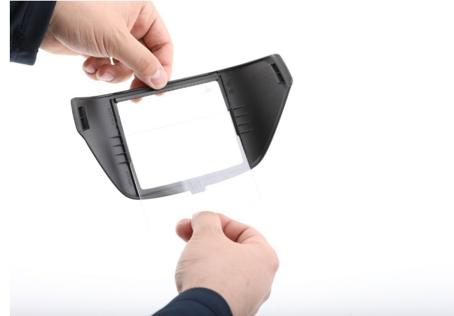
3.3 Fit a new protective lens.
