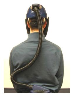
Make sure that the breathing hose runs down your back and is not twisted. You can adjust the angle of the helmet connection as required
