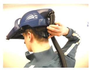
If necessary, adjust the width of the helmet using the knob located at the rear of the harness
