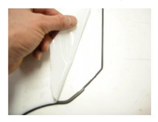
Remove the protective foils from the new visor.
