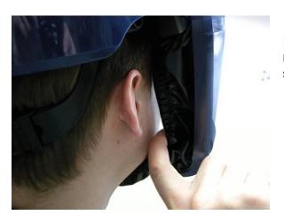
Insert a finger inside the face seal and move it along the length of the contact surface to check the fit.
