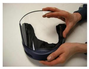
Fit the visor into the lower visor frame. Applying a little water to the seal will make fitting easier
