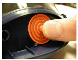
Press the new membrane securely on the pin. Carefully check that the membrane is fully in contact with the valve seat.
