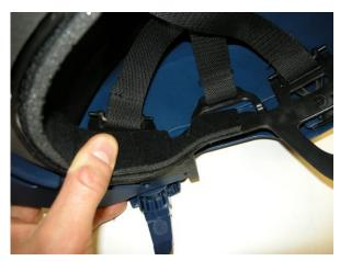
Fit the Velcro tape with the rough side towards the forehead strap and the groove facing upwards.
