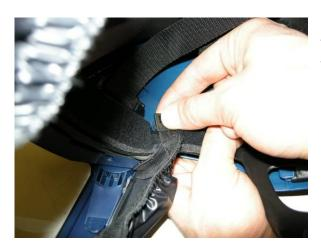
The sweatband is attached to the forehead strap by a Velcro tape.
