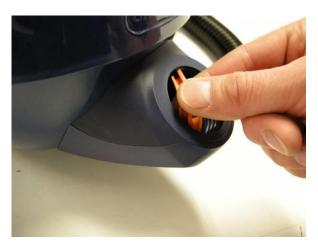
Remove the gasket from the flange.
